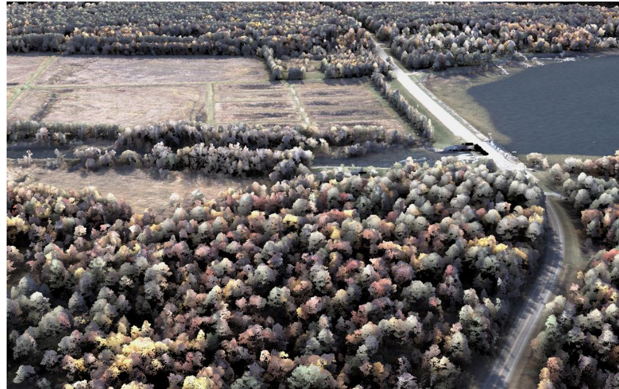
Lidar Point Cloud Colorized by Photo
